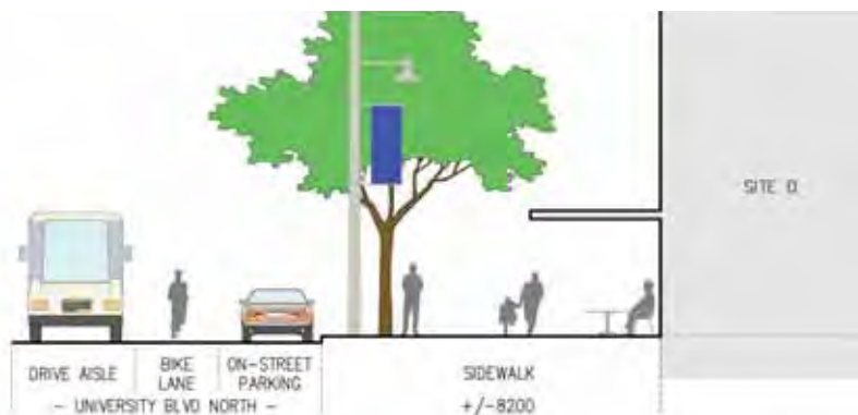
SITE D TYPICAL SECTION ALONG UNIVERSITY BOULEVARD
